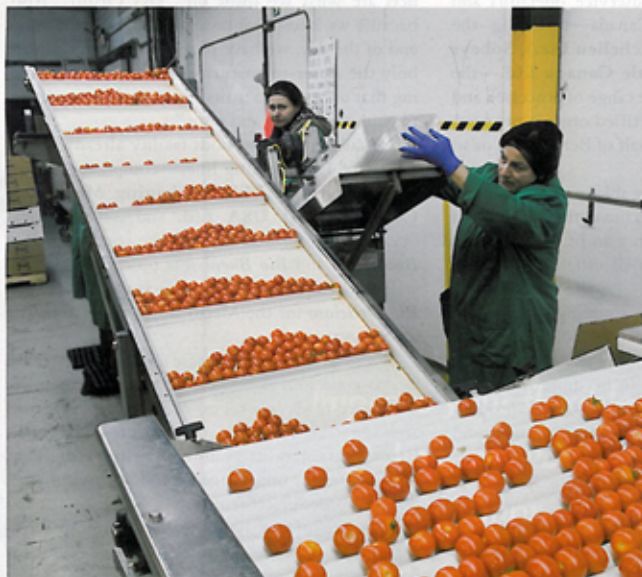
A worker places clear PET plastic clamshell containers manufactured by Reynolds Foods Packaging onto an inserter line as tomatoes move up the food-grade conveyor for packing.
