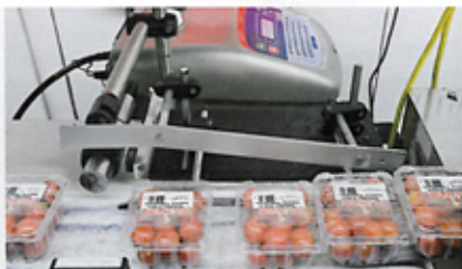
PET clamshell packages containing cherry tomatoes pass by the Linx model 7300FG continuous inkjet coder.
