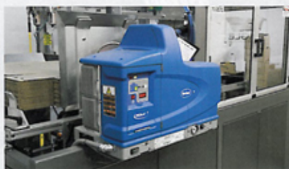
Part of the Vassoyo trayformer, a Nordson ProBlue 7 adhesive melter seals the corner flaps of the trays.
