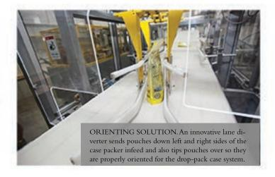
pouches the orientation needed for the drop-pack casing system that comes next in the line. Take 24-oz pouches, for example, which are packed 20 per case in five layers. The goal is to have the pouches, when they drop into their case, resting not on their gusseted bottoms but rather lying flat on their sides. Also required is that when they drop into the case four per layer, one layer has gusseted bottoms on the right and the next layer has gusseted bottoms on the left.
